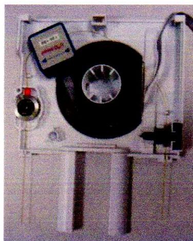
The C 4 D headstage in the Agilent cartridge. The round, silver UV detector cell can also be seen.
